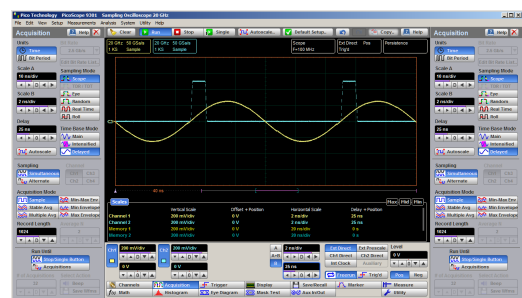
Delayed Timebase Mode
