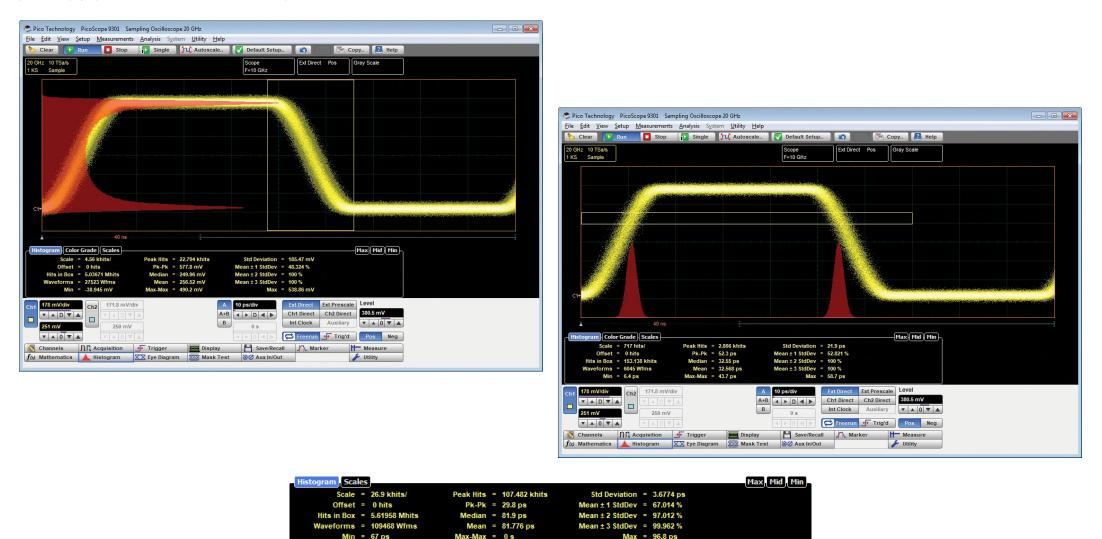
Histograms can be constructed on waveforms on either the vertical or horizontal axes. The most common use for a vertical histogram is measuring and characterizing noise and pulse parameters. A horizontal histogram is typically used to measure and characterize jitter.
