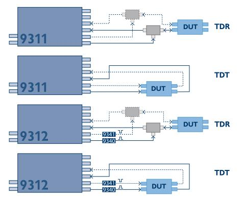
Connection diagrams: PicoScope 9311 and 9312 sampling oscilloscopes in use with devices under test (DUT) in TDR and TDT applications
