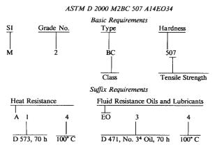
In this example, basic requirements for heat resistance and fluid resistance are superseded by suffix requirements. However, the basic requirement of 80 % for compression set, which is not included as a suffix requirement, is not superseded and therefore shall be met as specified in Table 6.
