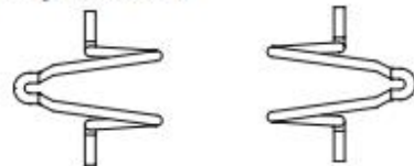
Fig.32 Connector retention clips to fasten the H15 connector to the rear plate; see fig. 29. HZZ01209-G consists of 2 clips.
